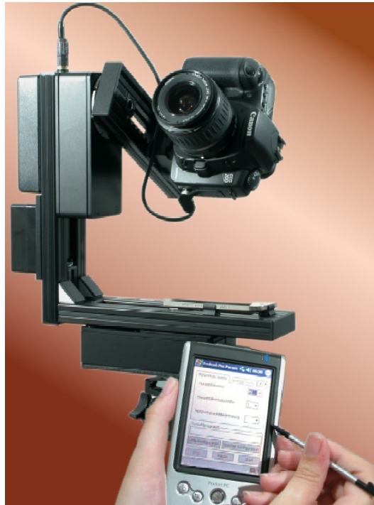
Figure 7.4: Automated panorama head. (Source: Wikipedia https://de.wikipedia.org/wiki/Panoramakamera#mediaviewer/File:Rodeon_vr_head_01.jpg )
