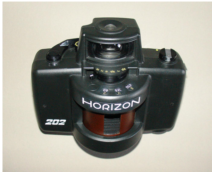
Figure 7.3: Zenit “Horizon 202” panorama camera with rotating lens for 35mm film. (Source: Wikipedia, “Horizon202” by BillC - Own Work. Licensed under CC BY-SA 3.0 via Wikimedia Commons - https://commons.wikimedia.org/wiki/File:Horizon202.jpg#mediaviewer/File:Horizon202.jpg )
