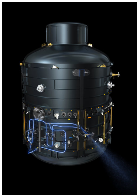
The cryogenic cooling system on-board the Herschel Space Telescope
