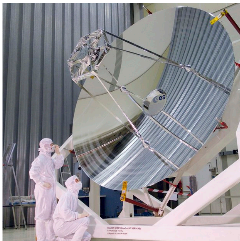
Mirror of the Herschel Space Telescope, during construction
