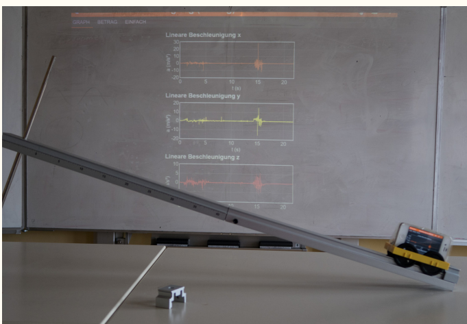
Figure 1. Inclined plane with mobile phone and phyphox app with remote control
