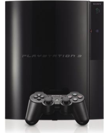
The Playstation 3: a Game Console, with Yellow Dog Linux running inside. 3.2 TerraFLOPS in the hands of children!
