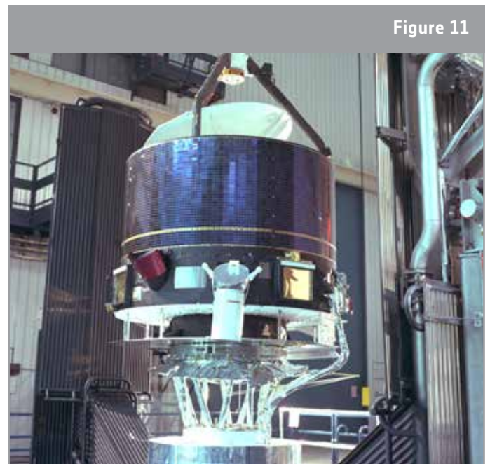
↑ Giotto ready for the solar simulation test. Copyright: ESA
