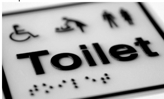
Fig. 6 Multiple layers of black UV-cured ink (source: https://www.fespa.com/news/features/how-to-print-3d-with-a-uv-digital-inkjet.html )
