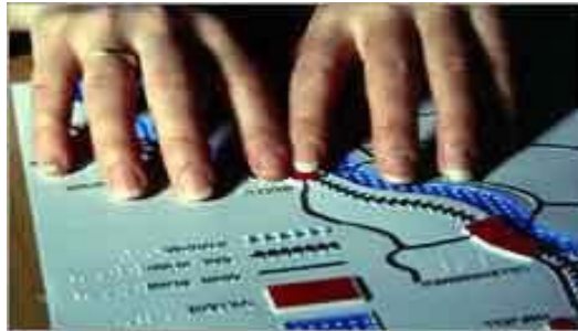
Fig. 5 Microcapsule or swell paper map (source: http://www.johngilltech.com/guidelines/tactile_maps.htm )
