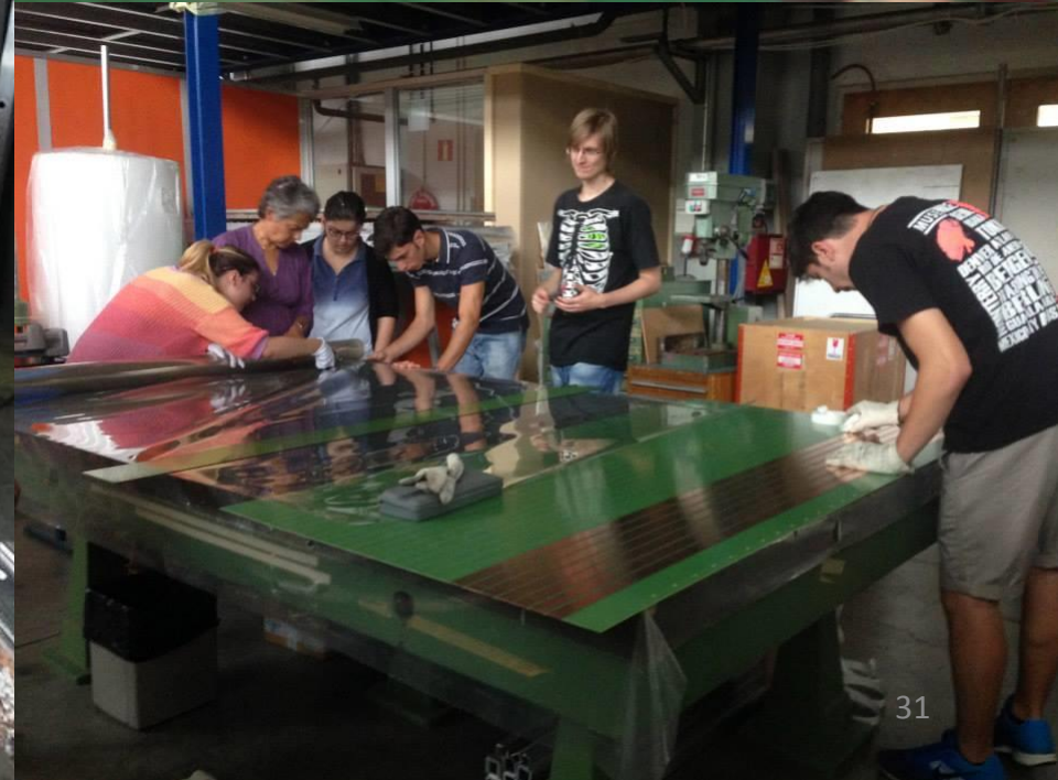
preparation of readout copper strips
