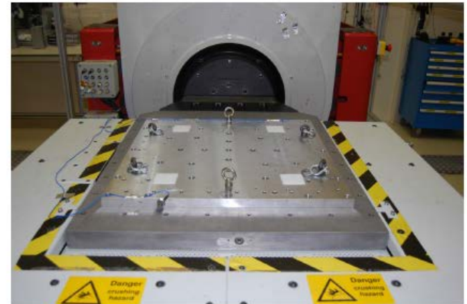
Figure 7: CTB Mounting Hardware Attached to Fixture on Slip Table (X axis configuration)
